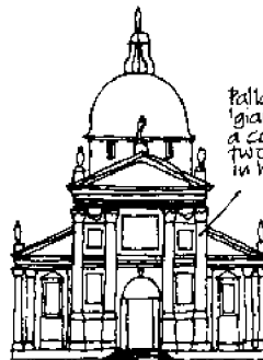
The church of San Giorgio Maggiore in Venice (1565) uses the giant order to emphasise the difference in scale between nave and aisles
