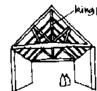
like the tie-beam roof, the king-post truss obscured the roof-shape
