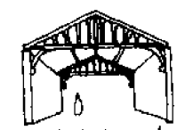
the tie-beam roof, often highly decorated, was appropriate to a low-pitched roof
